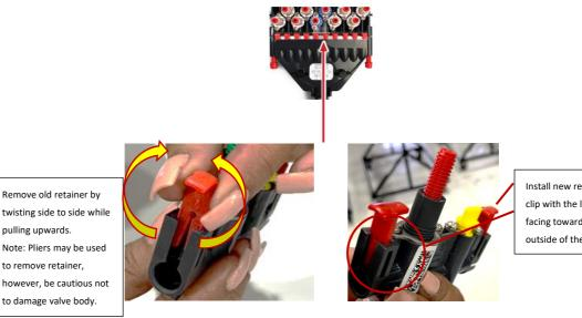
Install new retanier clip with the larger tab facing towards the outside of the valve
